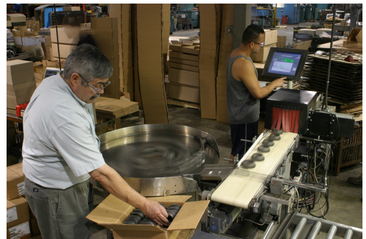
Figure 3. Fully automated system on plant floor, shown testing parts through acoustic chamber.
