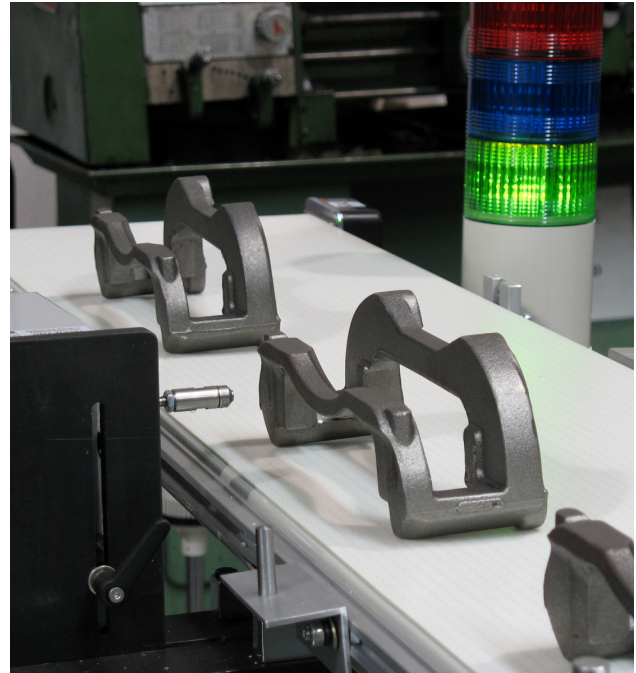
Figure 5. Ductile iron brake anchor on automated conveyor system.
